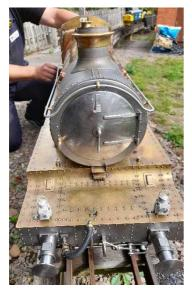
The loco frames were cut to Martin Evans design and later, where possible, works drawings provided the detail along with hundreds of photos of the prototype. Cookham Manor at Didcot provided the most authentic detail as it is still in the condition last used on British Railways.
